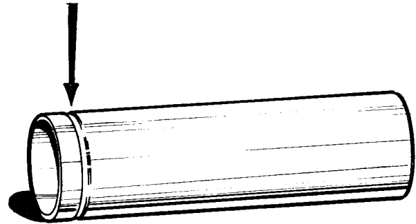
FIG. B.75. Sleeve pinion bush worn by oil seal.
