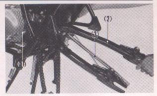
Fig. 5-75 (1) Rear fork pivot bolt
