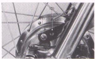
Fig. 5-13 (1) 8 mm bolt (U.B.S.) (2) Front brake stopper arm
