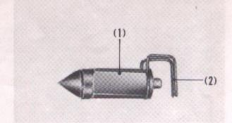
Fig. 2-19 (1) Float valve (2) Special clip
