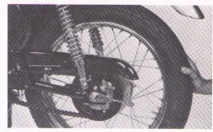
Fig. 4-6 Push rear wheel forward all the way
