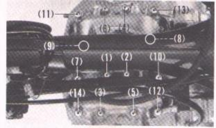
Fig. 4-38 Cylinder head cover tightening sequence
