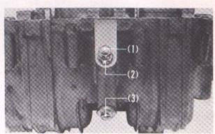
Fig. 4-77 (1) Tensioner setting bolt (2) Lock nut (3) Oil check bolt
