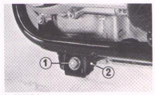
Fig. 36 (1) Bolt (2) Exhaust chamber damper
