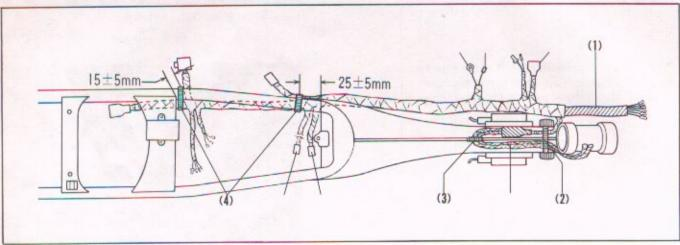
Fig. 5-90 (1) Wire harness (2) Wire harness clip A
