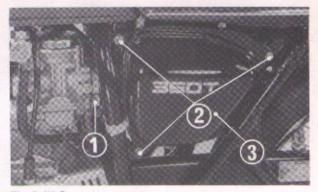
Fig. 6 (1) Screw (2) Nut (3) Air cleaner case cover
