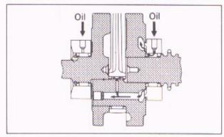
Fig. 2-14 Lubrication to crankshaft
