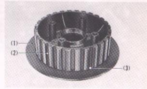
Fig. 4-55 (1) Clutch plate A (2) Clutch center (3) Stop ring
