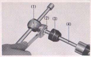
Fig. 5-79 (1) Upper joint (2) 9 mm lock nut (3) Stopper rubber
