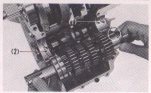
Fig. 4-94 (1) Dowel pin (2) Set ring
