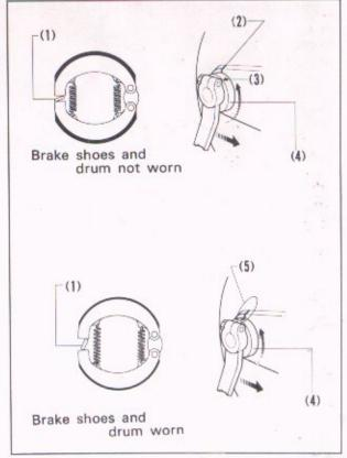
Fig. 2-23 (1) Brake cam
