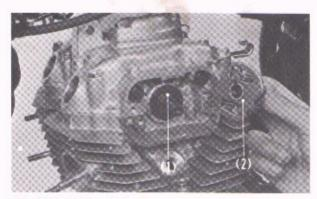
Fig. 4-39 (1) Dowel pin (2) Spark advancer
