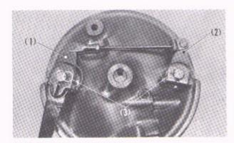
Fig. 5-18 (1) Front brake arm A (2) Front brake arm B
