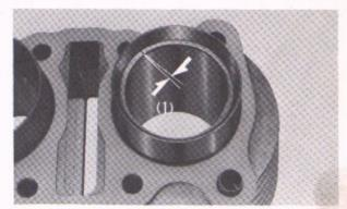
Fig. 4-27 (1) Piston ring gap
