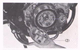
Fig. 4-57 (1) Clutch lifter joint piece (2) Clutch pressure plate
