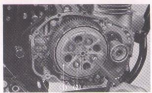
Fig. 4-51 (1) Clutch pressure plate
