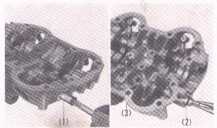
Fig. 4-16 (1) Right rocker arm shaft (2) Left rocker arm shaft
