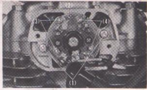
Fig. 3-8 (1) Base plate locking screws
