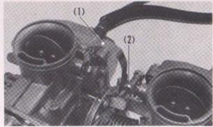
Fig. 4-105 (1) Connector joint (2) Bolt
