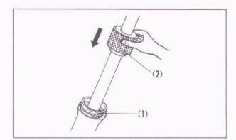
Fig. 5-61 (1) Oil seal (2) Fork seal driver
