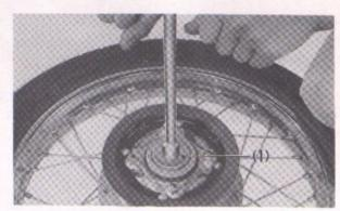
Fig. 5-39 (1) Bearing retainer wrench
