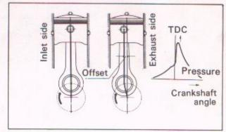
Fig. 2-5 Piston pin offset
