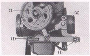
Fig. 4-114 (1), (2) Clips (3) Holding bolt (4) Throttle lever (5) Adjusting holder
