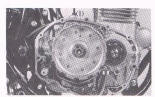
Fig. 4-53 (1) Clutch outer
