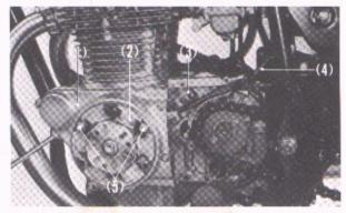
Fig. 4-42 (1) Left crankcase cover (3) Neutral switch lead (2) Stator
