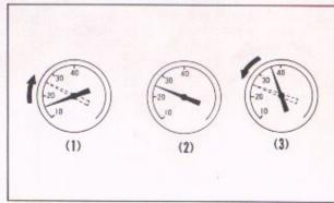
Fig. 3-15 (1) High speed (throttle too open)
