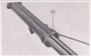
Fig. 5-58 (1) 48 mm internal snap ring
