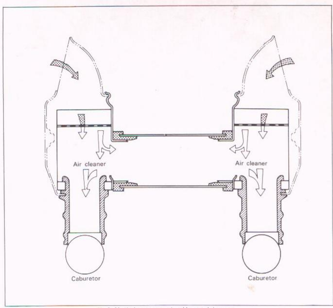
Fig. 2-28 Air cleaners communicated by central air passage
