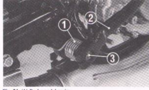
Fig. 21 (1) Brake pedal spring
