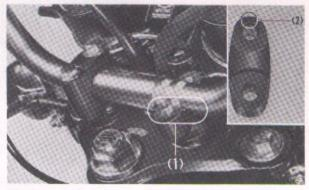
Fig. 5-53 (1) Punch mark on handlebar pipe and top of lower holder
