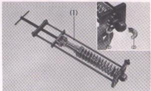
Fig. 5-76 (1) Rear shock absorber compressor (2) Spring seat stoppers
