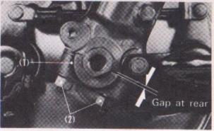
Fig. 5-19 (1) Front axle holder (2) 8 mm nut
