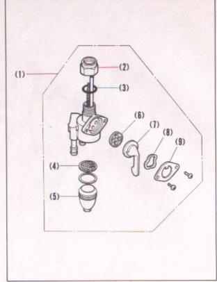
Fig. 5-84 (1) Fuel valve assy.
