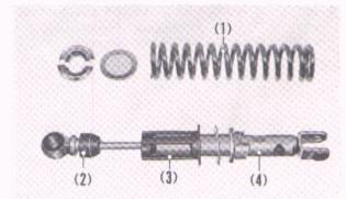
Fig. 5-78 (1) Rear shock absorber spring
