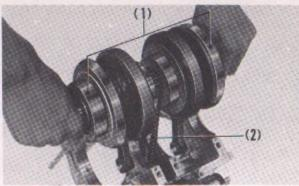
Fig. 4-100 (1) Crankshaft (2) Cam chain
