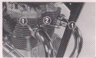
Fig. 37 (1) Joint nut (2) Exhaust pipe joint
