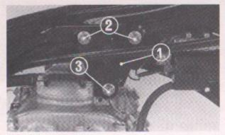
1 Remove the UBS nuts (2), (3) and (4). The left foot peg will be removed when the nut (3) is removed. Draw out the bolt by removing the nut (4).
