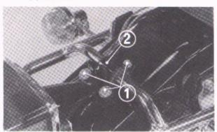
Fig. 25 (1) Bolt (2) Rear fender stay
