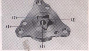
Fig. 2-8 (1) Oil pump body (2) Outer rotor
