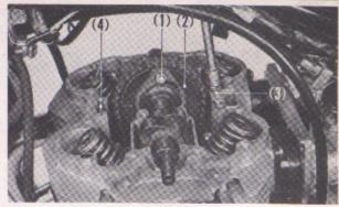
Fig. 4-17 (1) Fixing bolt
