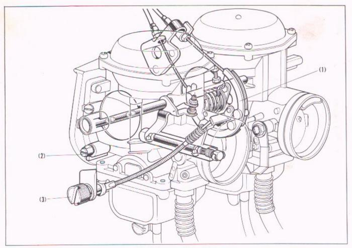
Fig. 2-20 (1) Throttle lever
