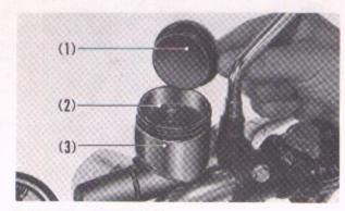
Fig. 3-30A (1) Diaphragm (2) Level mark (3) Reservoir
