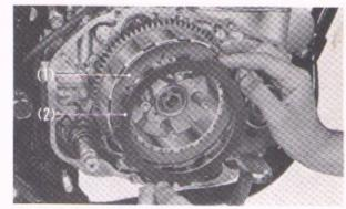
Fig. 4-56 (1) Clutch plate B (2) Friction disc
