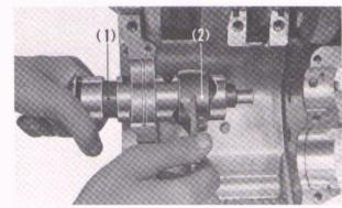
Fig. 4-89 (1) Gearshift drum (2) Gearshift fork B
