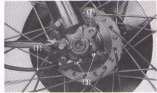
Fig. 5-2 (1) Speedometer cable (2) Axle holder
