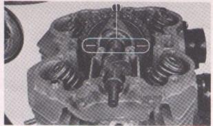
Fig. 4-36 (1) Matching lines on cam sprocket
