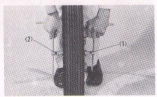
Fig. 5-16 (1) Front axle sleeve (2) Front wheel axle
