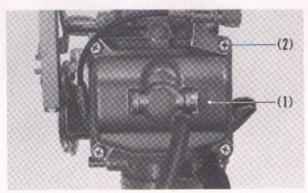
Fig. 4-117 (1) Float chamber body (2) Screw (longer)
