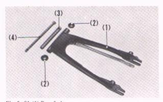
Fig. 5-81 (1) Rear fork (2) Dust seal caps (3) Rear fork center collar
