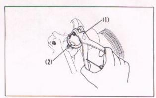
Fig. 5-29 (1) Snap ring pliers (2) Snap ring
