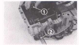
Fig. 14 (1) Kick starter ratchet (2) Kick starter spindle
