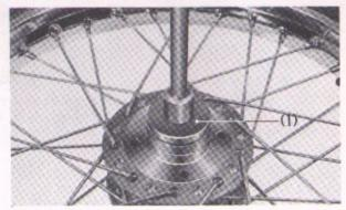
Fig. 5-5 (1) Bearing retainer wrench
