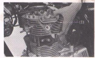
Fig. 4-19 (1) Cylinder head
