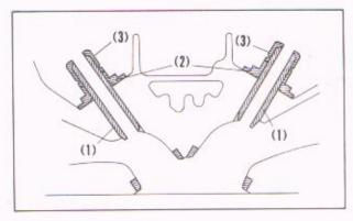
Fig. 2-2 (1) Valve guide (2) Spring seat (3) Stem seal
