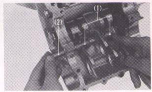
Fig. 4-92 (1) Gearshift fork A (2) Gearshift fork guide shaft
