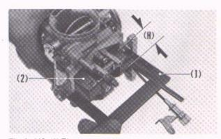
Fig. 4-119 (1) Float level gauge (2) Float
