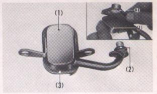
Fig. 4-69 (1) Oil filter screen (2) O-ring
