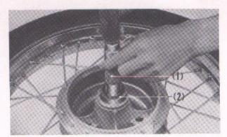
Fig. 5-42 (1) Driver handle (2) Race driver attachment
