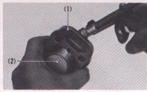
Fig. 5-28 (1) Caliper A (2) Piston
