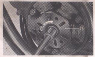
Fig. 3-4 (1) Generator rotor
