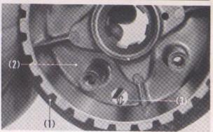
Fig. 4-54 (1) Clutch plate A (2) Clutch center
