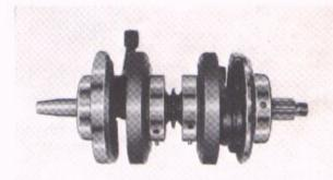
Fig. 2-13 Crankshaft
