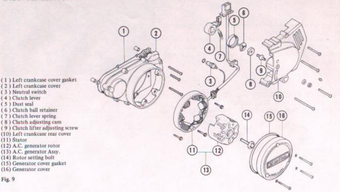
The construction of the generator is as shown in Fig. 9 immediately above. The starting mechanism is eliminated.
