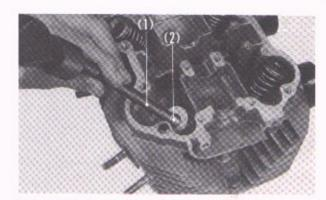
Fig. 4-28 (1) Valve guide remover (2) Valve guide
