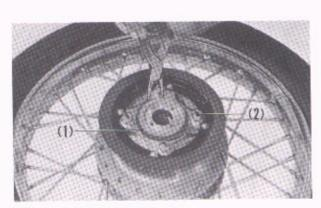
Fig. 5-44 (1) 69 mm snap ring (2) 10 mm UBS nut
