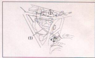
Fig. 4-4 (1) Starting motor cable (2) Starter magnetic switch
