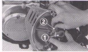
Fig. 10 (1) Clutch lever (2) Clutch cable end
