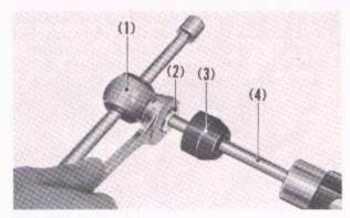
Fig. 5-77 (1) Upper joint (2) 9 mm lock nut
