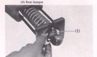
Fig. 5-80 (1) Spring seat stops (2) Rear shock absorber compressor
