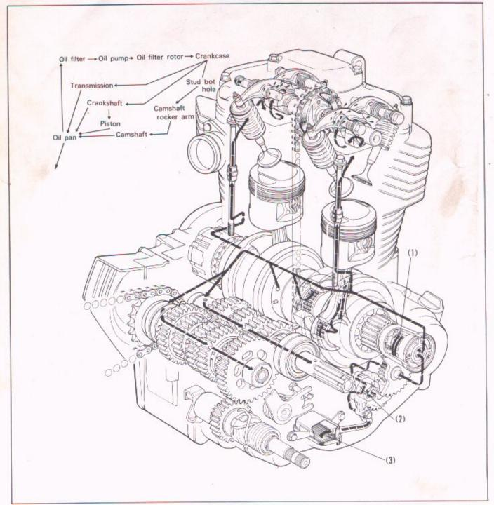
Fig. 2-7 Lubricating oil circuit
