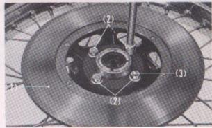
Fig. 5-4 (1) Brake disc (2) 8 mm UBS nuts (3) Bolts
