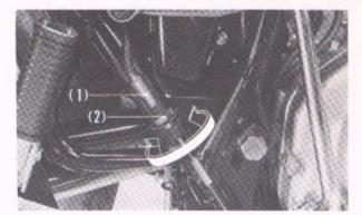
Fig. 6-29 (1) Rear stop switch (2) Adjusting nut
