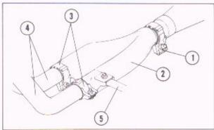
Fig. 40 (1) Muffler clamp
