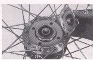
Fig. 5-9 (1) O-ring (2) Gear box retainer
