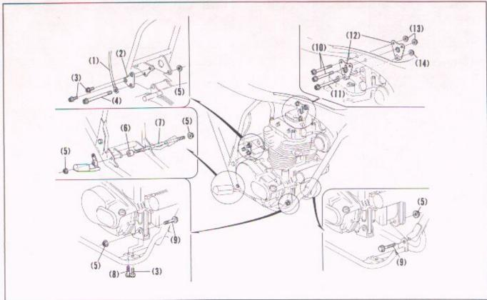
Fig. 4-2 (1) Battery ground cable (2) Engine hanger plate (3) 8 x 14 UBS bolt
