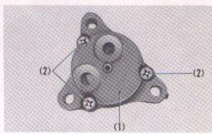
Fig. 4-62 (1) Oil pump body
