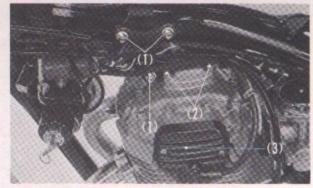
Fig. 4-13 (1) Nuts (2) Bolts (3) Point cover
