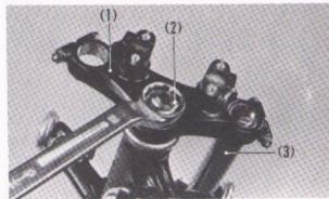
Fig. 5-71 (1) Fork top bridge (2) Steering stem
