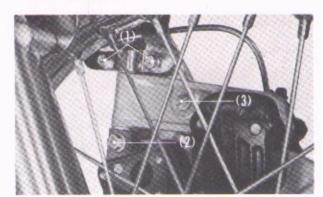
Fig. 5-23 (1), (2) Bolts (3) Adjusting bolt
