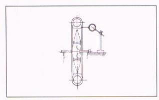
Fig. 5-6 Checking wheel rim for runout
