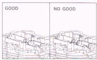
Fig. 4-24 Checking the surface of the camshaft journal
