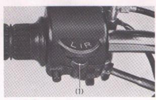
Fig. 6-32 Turn signal switch
