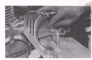
4-41 (1) Clutch lever (2) Clutch cable end
