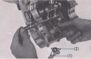
Fig. 4-87 (1) Shift drum stopper (2) Shift drum stopper spring
