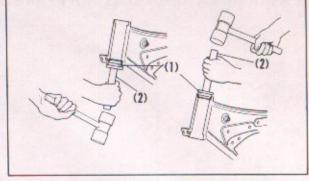
Fig. 5-69 (1) Race driver attachment (2) Driver handle
