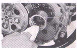
Fig. 3-24 (1) Oil filter rotor
