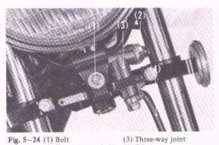
Fig. 5-24 (1) Bolt (4) Oil pipe (2) Front stop switch
