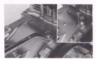
Fig. 4-85 (1) 12 mm lock washer (2) Shift drum guide screw
