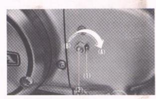
Fig. 3-19 (1) Clutch adjuster lock nut (2) Clutch adjuster
