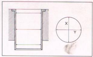
Fig. 4-26 Measure the cylinder bore
