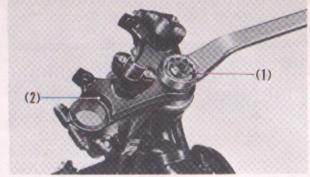
Fig. 5-65 (1) Steering stem nut (2) Fork top bridge
