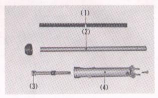
Fig. 5-59 (1) Front shock absorber spring
