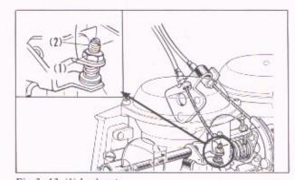
Fig. 3-13 (1) Lock nut (2) Adjusting screw
