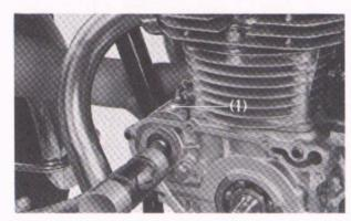
Fig. 4-45 (1) Starting motor
