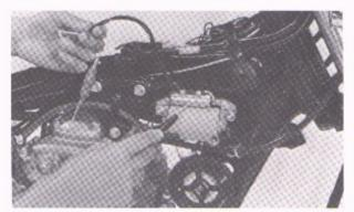
Fig. 6-14 Condenser checking
