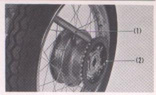
Fig. 5 -38(1) Wood block (2) Final driven sprocket
