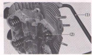
Fig. 4-22 (1) Valve spring compressor (2) Valve cotters
