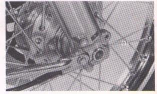
Fig. 3-40 (1) Front fork drain plug
