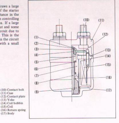
Fig. 6-24 (1) Stopper (2) Stopper holder (3) Washer (4) Roller A (5) Contact spring (6) Flat washer
