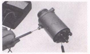
Fig. 6-23 Checking stator coil
