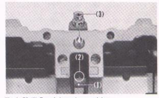
Fig. 4-78 (1) Cam chain tensioner push bar
