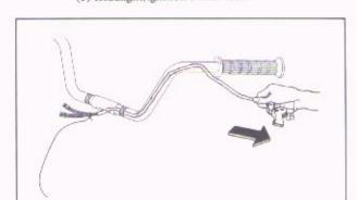
Fig. 5-51 Pulling switch lead
