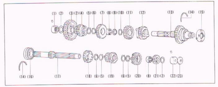
Fig. 4-93 (1) 20 mm needle bearing
