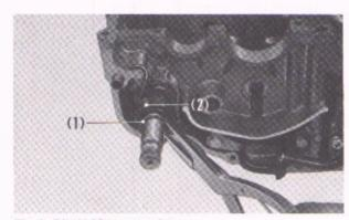
Fig. 4-74 (1) 18 mm snap ring (2) Kick starter spring
