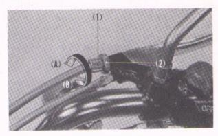
Fig. 3-33 (1) Front brake cable adjuster (2) Lock nut
