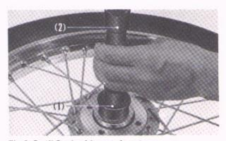
Fig. 5-7 (1) Bearing driver attachment
