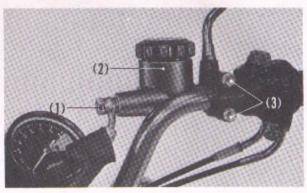
Fig. 5-22 (1) Oil bolt (2) Master cylinder assembly (3) Bolts
