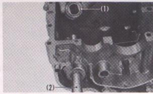
Fig. 4-80 (1) Kick starter ratchet (2) Kick starter spindle
