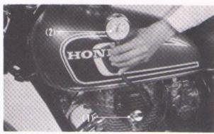
Fig. 3-45 (1) Compression gauge attachment (2) Compression gauge
