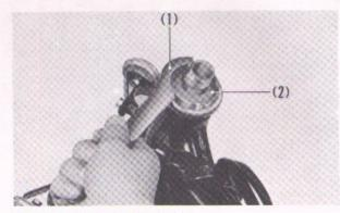
Fig. 5-66 (1) 46 mm pin spanner (2) Steering head top thread
