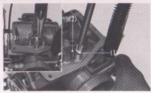
Fig. 4-113 (1) Screw (2) Valve seat plate (3) Valve seat
