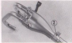
Fig. 38 (1) Exhaust pipe joint (2) Muffler band
