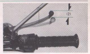
Fig. 3-31 (1) Front brake lever (2) Lever free play
