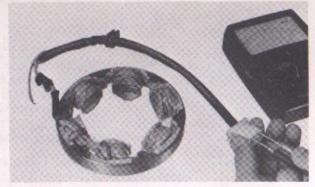
Fig. 6-4 Stator continuity test
