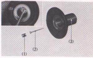
Fig. 4-110 (1) Needle jet screw (2) Jet needle (3) Vacuum piston
