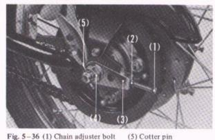
Fig. 5-36 (1) Chain adjuster bolt
