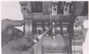
Fig. 4-88 (1) Guide pin clip (2) Guide pin
