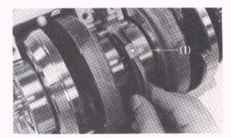
Fig. 4-99 (1) Cam chain tensioner arm
