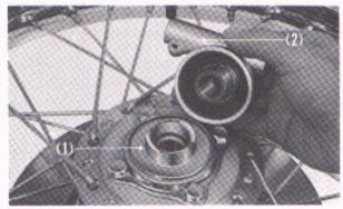
Fig. 5-10 (1) Gear box retainer (2) Speedometer gear box
