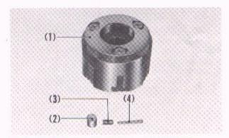
Fig. 4-46 (1) Starting clutch outer
