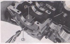
Fig. 4-76 (1) Oil separators (2) Oil separator setting bar
