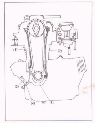
Fig. 2-6 (1) Cam chain slipper
