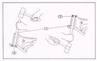
Fig. 5-67 (1) Ball race remover (2) Ball race
