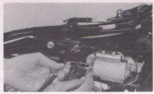
Fig. 6-11 Ignition coil continuity test
