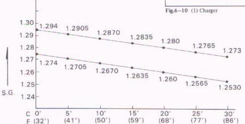
Relationship between atmospheric temperature and specific gravity
