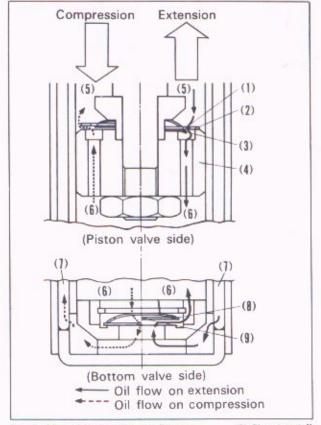
Fig. 2-27 (1) Orifice (I) (4) Piston (7) Chamber "c" (5) Chamber "a" (2) Valve "A" (8) Bottom valve (6) Chamber "b" (3) Valve "B" (9) Orifice (II)
