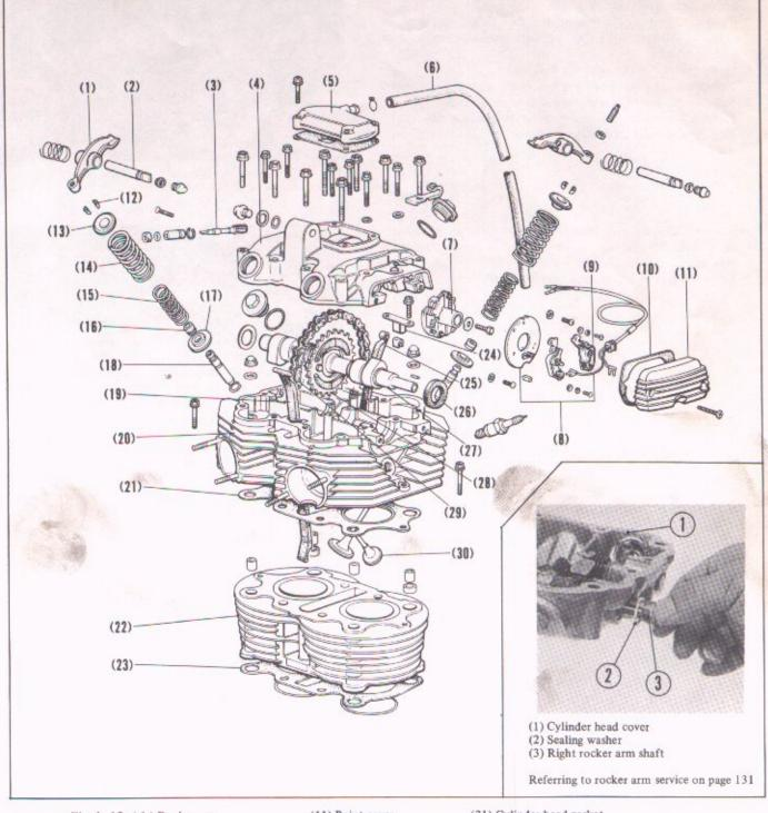
Fig. 4-12 (1) Rocker arm (2) Rocker arm shaft (L)
