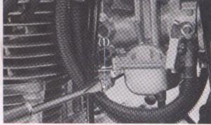
Fig. 3-10 (1) Throttle stop screw
