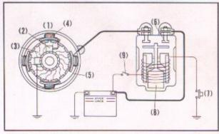
Fig. 6-21 (1) Starting motor (6) Starting magnetic switch
