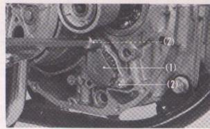
Fig. 4-61 (1) Oil pump assembly (2) Bolt
