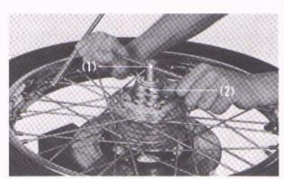
Fig. 5-3 (1) Front wheel axle (2) Speedometer gear box
