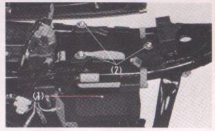
Fig. 5-87 (1) Battery box (2) Bolts
