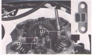
Fig. 4-37 (1) Cam chain tensioner holder
