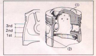
Fig. 2-4 Sectional view of piston
