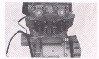
Fig. 4-71 (1) Upper crankcase tightening bolt
