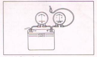
Fig. 6-2 Battery charging test
