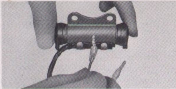
Fig. 6-20. Short-circuiting of the condenser
