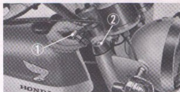
① Front fork bolt ② Oil filler opening
