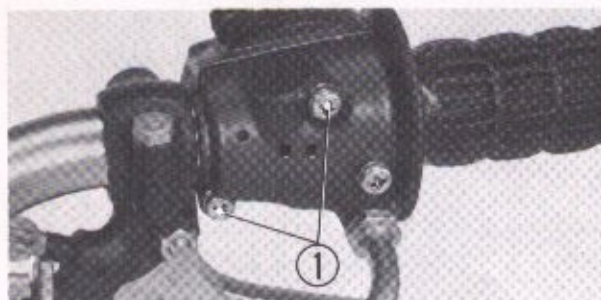
① Switch mounting screw Fig. 9-2.
