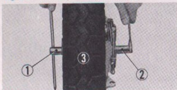
① Front wheel axle ② Front wheel axle sleeve ③ Front wheel tire
