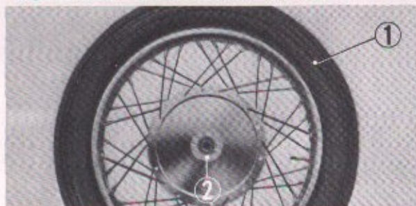
① Front wheel tire ② Oil-seal
