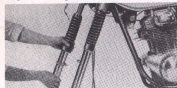
Fig. 5-27. Installing the front fork into the steering
