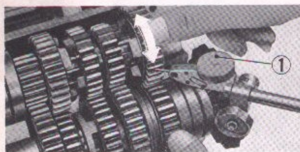
Fig. 4-109. Measuring the gear backlash
