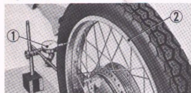
① Dial gauge ② Front wheel rim
