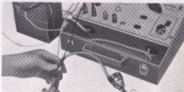
Fig. 6-80. Continuity test of the ignition switch
