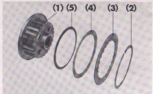
**Fig. 3-32** (1) Clutch center (2) Set ring
