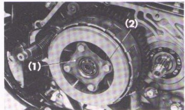
Fig. 3-26 (1) Clutch lifter plate
