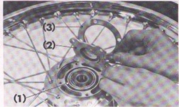
Fig. 4-9 (1) O-ring (2) Gear box retainer
