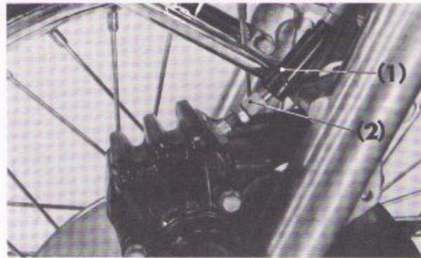
Fig. 4-12 (1) Cable boot (2) Cable adjusting bolt
