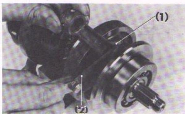
Fig. 3-62 (1) Connecting rod (2) Feeler gauge
