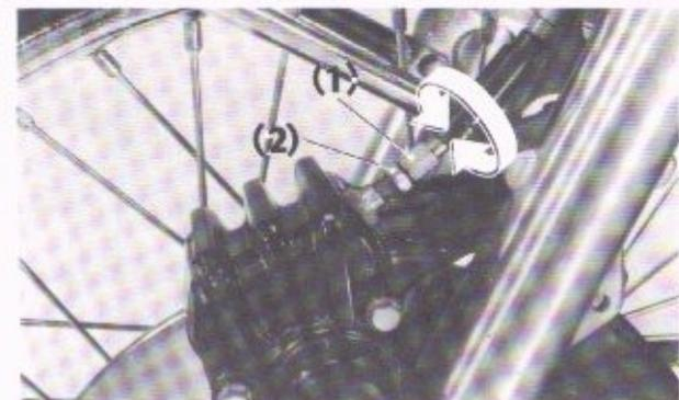
Fig. 4-29 (1) Cable adjusting bolt (2) Lock nut
