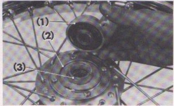
Fig. 4-4 (1) Speedometer gear box
