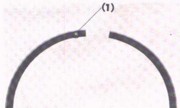
Fig. 3-14 (1) Piston ring top marking
