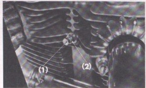
Fig. 2-13 (1) Tensioner setting bolt
