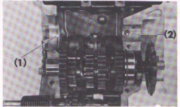
Fig. 3-49 (1) Ball bearing set ring
