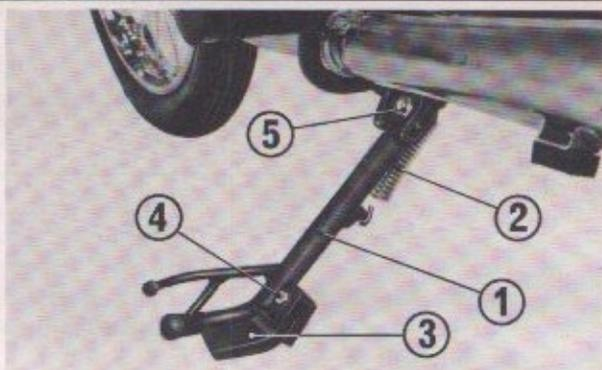
Fig. T-4 (1) Side stand bar (2) Spring
