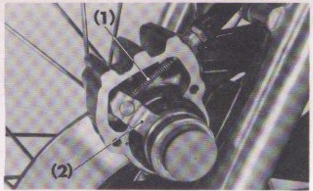
Fig. 4-14 (1) Brake cable (2) Brake arm
