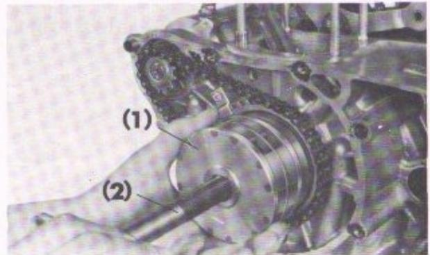
Fig. 3-58 (1) Generator rotor (2) Rotor puller
