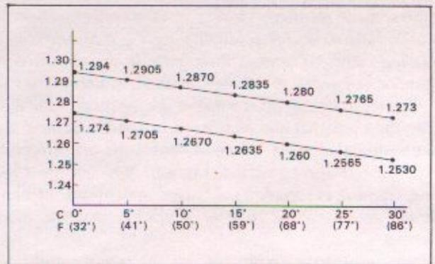
Fig. 5-18 Relationship between atmospheric temperature and specific gravity
