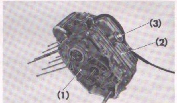
Fig. 3-39 (1) Upper crankcase (2) Lower crankcase
