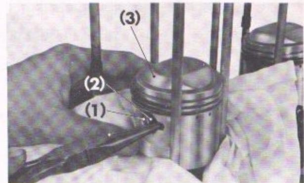
Fig. 3-9 (1) Piston pin clip
