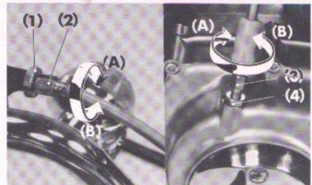
Fig. 2-10 (1) Clutch cable upper adjuster lock nut
