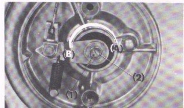
Fig. 2-11 (1) Clutch adjuster
