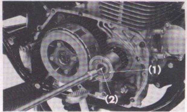
Fig. 3-23 (1) Oil filter cap
