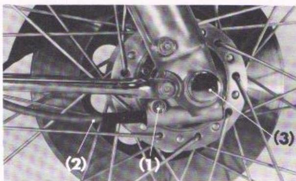
Fig. 4-2 (1) Setting screw (2) Speedometer cable
