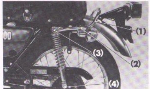
Fig. 4-70 (1) Rear pipe (2) Rear pipe bolt
