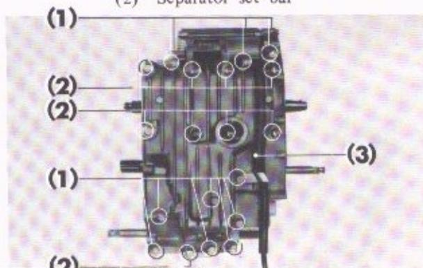
Fig. 3-66 (1) 6mm bolt (2) 8mm bolt
