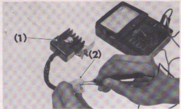
Fig. 5-14 (1) Silicon diode rectifier (2) Connector
