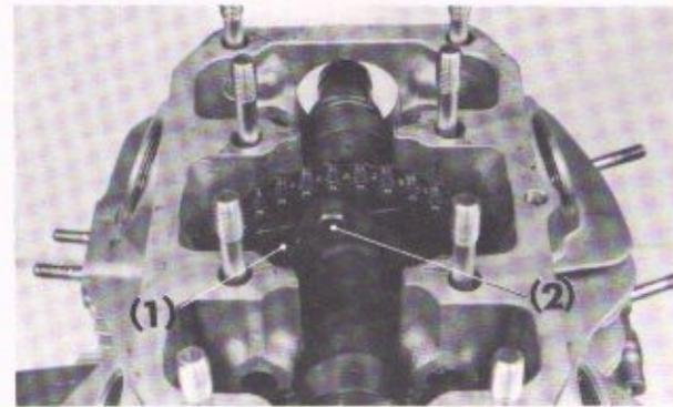
Fig. 3-5 (1) Cam sprocket (2) Knock bolt
