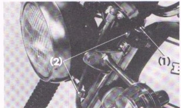
Fig. 4-64 (1) Front fork bolt (2) Fork attaching bolt
