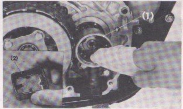
Fig. 2-28 (1) Oil filter rotor
