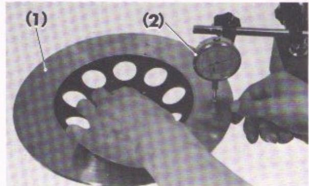
Fig. 4-6 (1) Brake disc (2) Dial gauge
