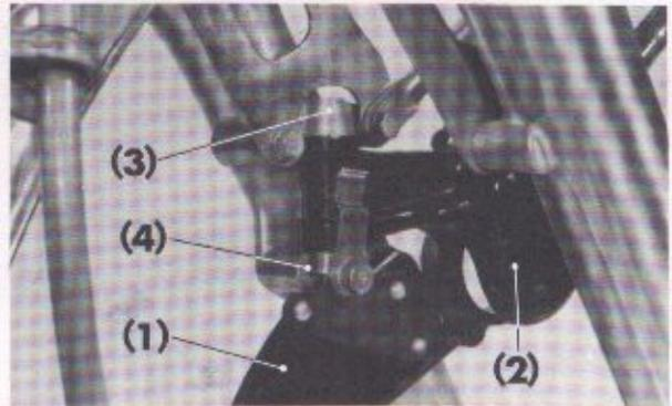
Fig. 4-19 (1) Disc cover (2) Caliper body
