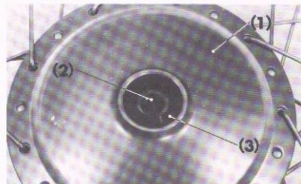
Fig. 4-38 (1) Front wheel hub (2) Ball bearing
