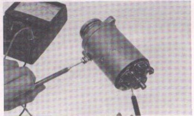
Fig. 5-24 Checking stator coil
