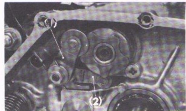
Fig. 3-45 (1) Gear shift drum stopper arm
