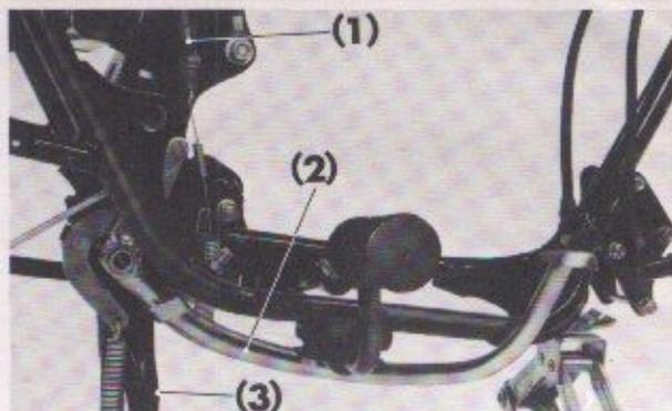
Fig. 4-79 (1) Stop switch (2) Brake pedal
