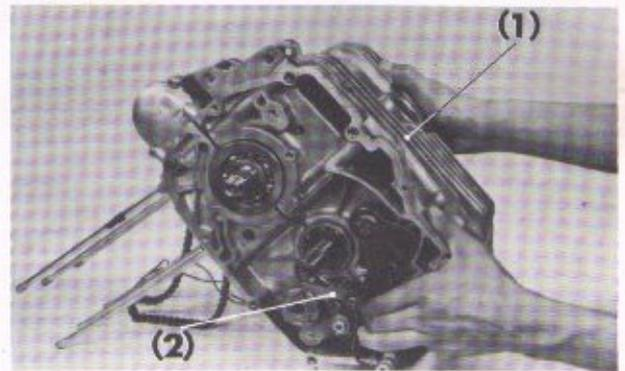
Fig. 3-47 (1) Lower crankcase (2) Gear shift arm
