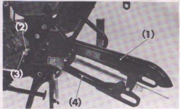
Fig. 4-72 (1) Drive chain case (3) Pivot bolt
