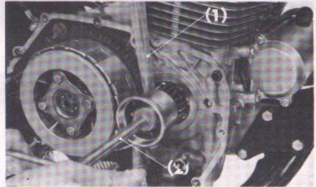
Fig. 3-24 (1) Piece of soft metal bar
