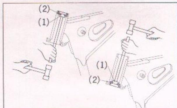
Fig. 4-80 (1) Ball race remover (2) Ball race
