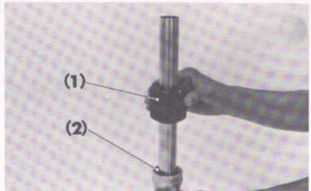
Fig. 4-67 (1) Fork seal driver (2) Oil seal
