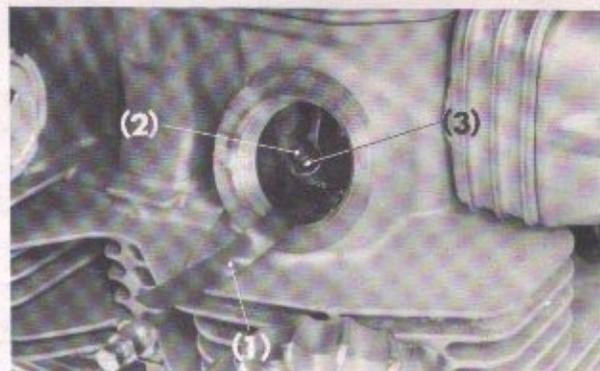
Fig. 2-2 (1) Feeler gauge (2) Tappet adjusting screw (3) Lock nut
