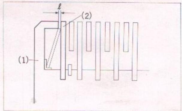
**Fig. 3-33** (1) Clutch center (2) Clutch plate B
