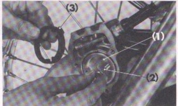
Fig. 4-15 (1) Pad A (2) 6mm bolt
