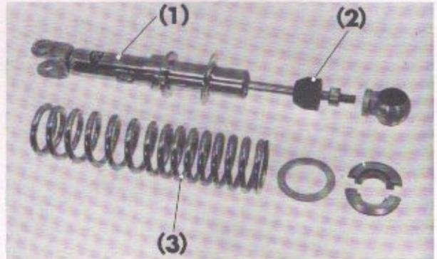
Fig. 4-73 (1) Rear shock absorber
