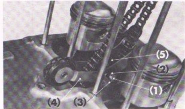
Fig. 3-55 (1) Bolt (2) Snap ring (3) Guide roller pin (4) Chain tensioner roller (5) Guide roller
