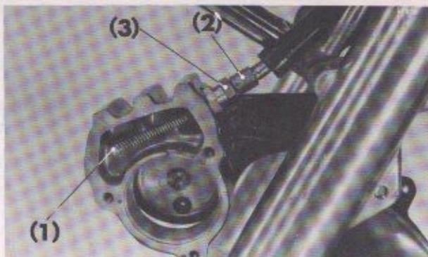
Fig. 4-22 (1) Cable end (2) Adjusting bolt
