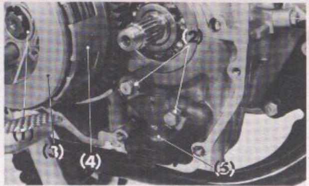
Fig. 3-27 (1) Snap ring (2) Lock washer
