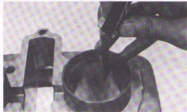
Fig. 3-13 Measuring piston ring end gap
