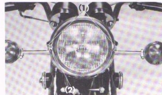
Fig. 2-39 (1) Headlight mounting bolt
