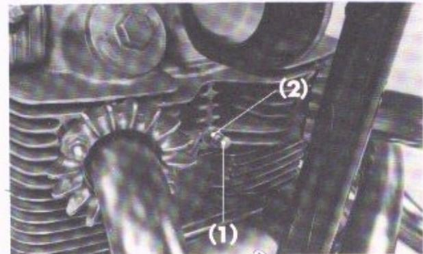
Fig. 3-56 (1) Chain tensioner setting bolt (2) Lock nut
