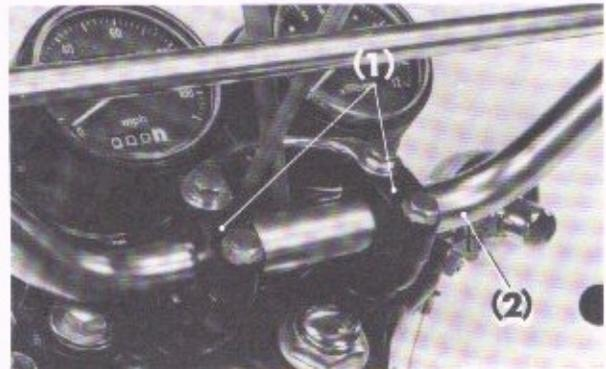
Fig. 4-50 (1) Upper handlebar holder (2) Steering handlebar
