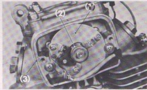
Fig. 3-3 (1) Contact breaker base plate
