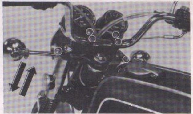
Fig. 2-36 (1) Checking front suspension
