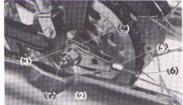
Fig. 2-34 (1) Cotter pin (2) Rear axle nut
