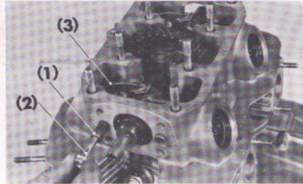
Fig. 3-4 (1) Rocker arm shaft
