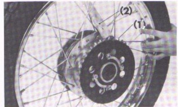
Fig. 4-43 (1) Final driven sprocket (2) Piece of wood
