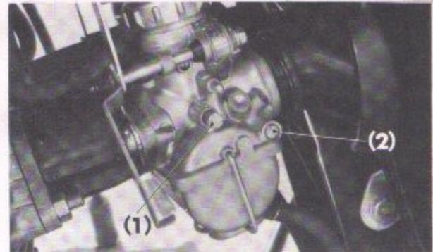
Fig. 2-6 (1) Stop screw (2) Air screw
