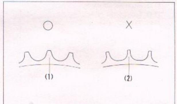
Fig. 4-45 Checking wear on final driven sprocket
