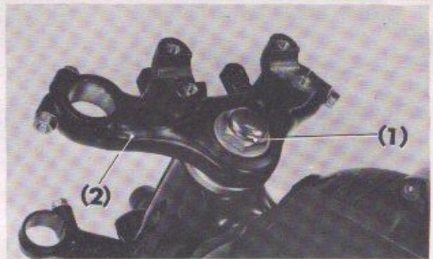
Fig. 4-58 (1) Steering stem nut
