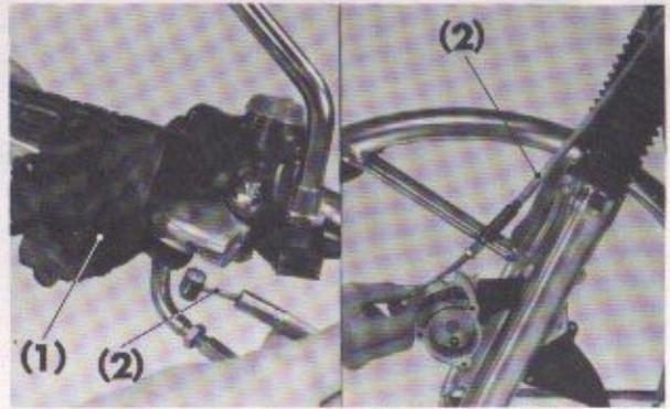
Fig. 4-18 (1) Lever boot (2) Brake cable
