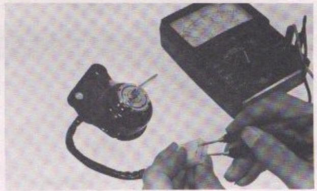
Fig. 5-29 Checking main switch for continuity
