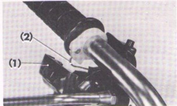
Fig. 4-49 (1) Switch (2) Throttle cable
