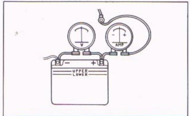
Fig. 5-10 Charging test
