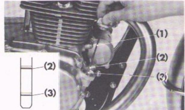
Fig. 2-14 (1) Filler cap (2) Upper level mark
