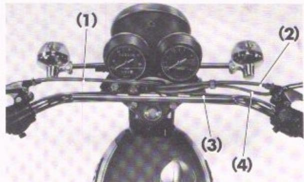
Fig. 4-54 (1) Clutch cable (2) Brake cable
