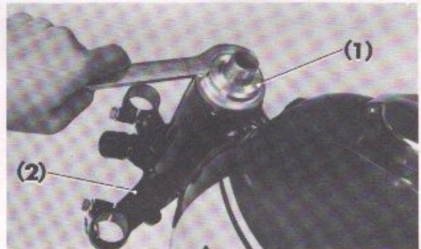
Fig. 4-59 (1) Steering head top thread
