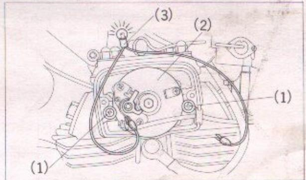
Fig. 2-5 (1) Base plate locking screw (2) Base plate (3) Test lamp
