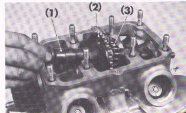
Fig. 3-6 (1) Camshaft (2) Sprocket
