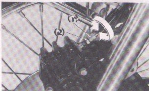
Fig. 2-17 (1) Front brake cable adjusting bolt
