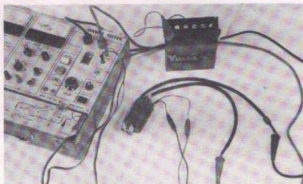
Fig. 5-4 Checking ignition coil performance
