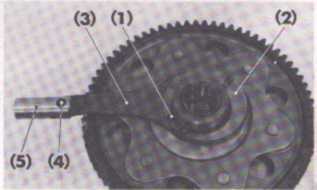
Fig. 3-28 (1) Snap ring (2) Side washer
