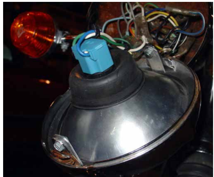
Headlamp with H-4 fixture installed. Note the two aluminum stanchions bolted into the bezel's old pivot stanchions. Also note the socket wiring arrangement.
