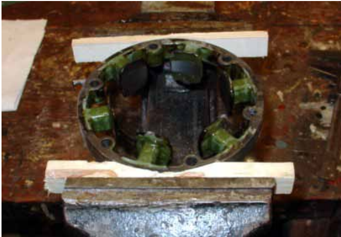
Empty stator held in vise with radiused wood slats.
