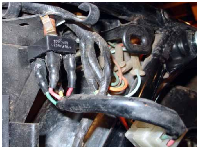
New Rectifier Installed in Place of Old One. RadioShack 276-1185
