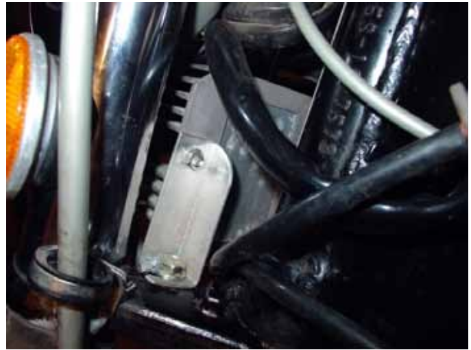
Back side of voltage regulator. Mounted with \frac{3}{4} inch aluminum angle.
