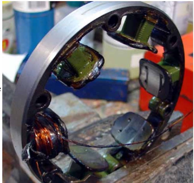
Stator being de-wound.
