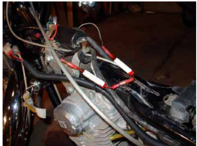
Ignition resistors wired in, but not folded in to fit within the gas tank enclosure.
