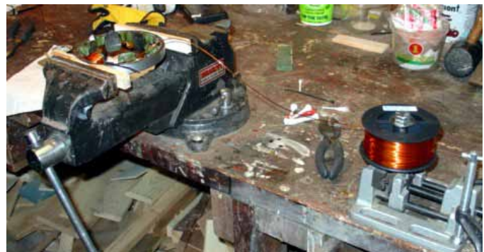
Winding station with stator held in vise, and wire spool held in stand clamped to workbench.
