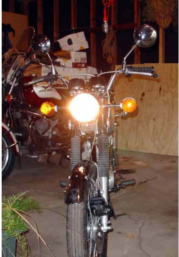
It works! With H-4 headlamp on low-beam, system voltage achieves 13.0 V at 1800 indicated rpm.
