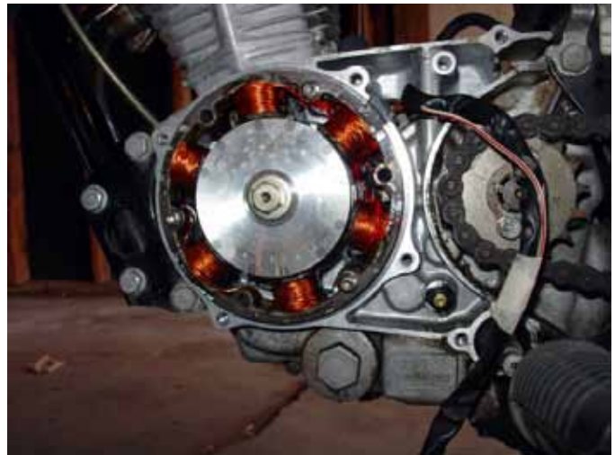
New stator installed in the engine.
