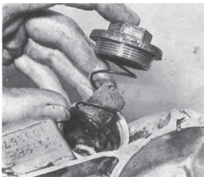
Strainer is easily removed for cleaning
